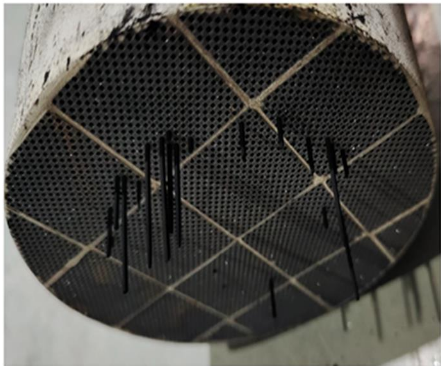
气流吹扫孔道/air sweeps
