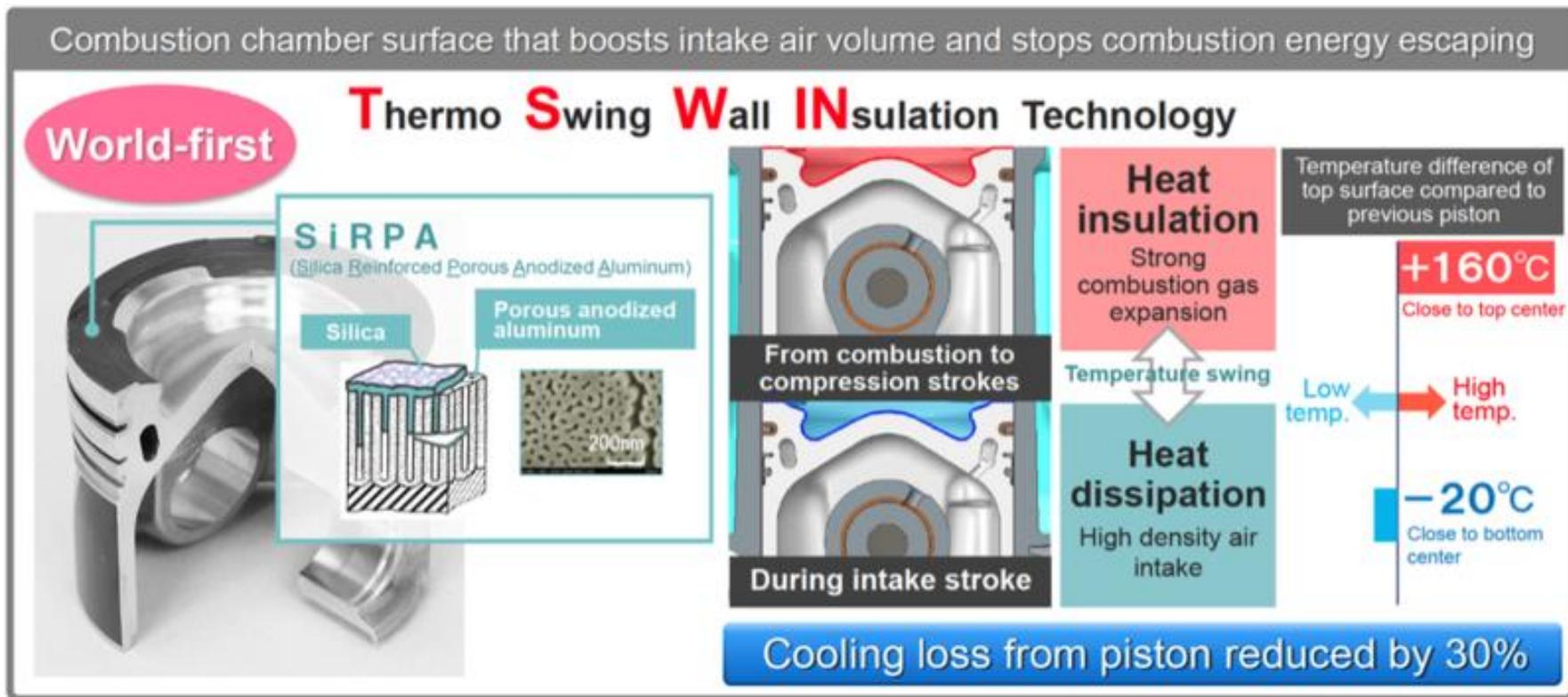
Thermal-Swing Wall Insulation Technology (TSWIN) in spark-ignition and compression-ignition engines was evaluated through computation. The rate of improvement of the thermal efficiency increases as the thermal conductivity and volumetric heat capacity fall.
