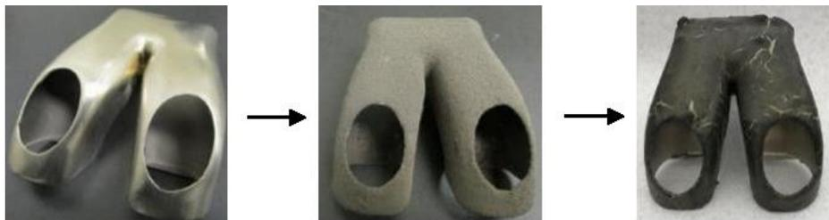
Nickel exhaust port shells were coated and sintered, then placed in cylinder head mold for casting.
