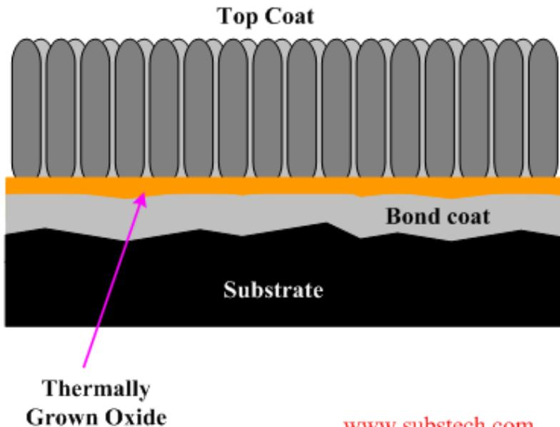
**Metallic Bond Coat** with a thickness of about 0.004" (0.1 mm).
