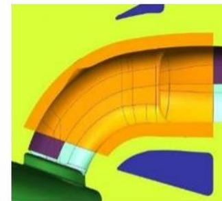
Model of a liner cast into the exhaust port
