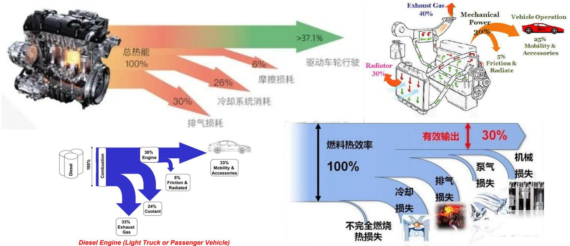
Currently, a high level of the heat energy produced in internal combustion engines, whether gasoline or diesel, is wasted by heat loss in the forms of exhaust, coolant and mechanical energy.
