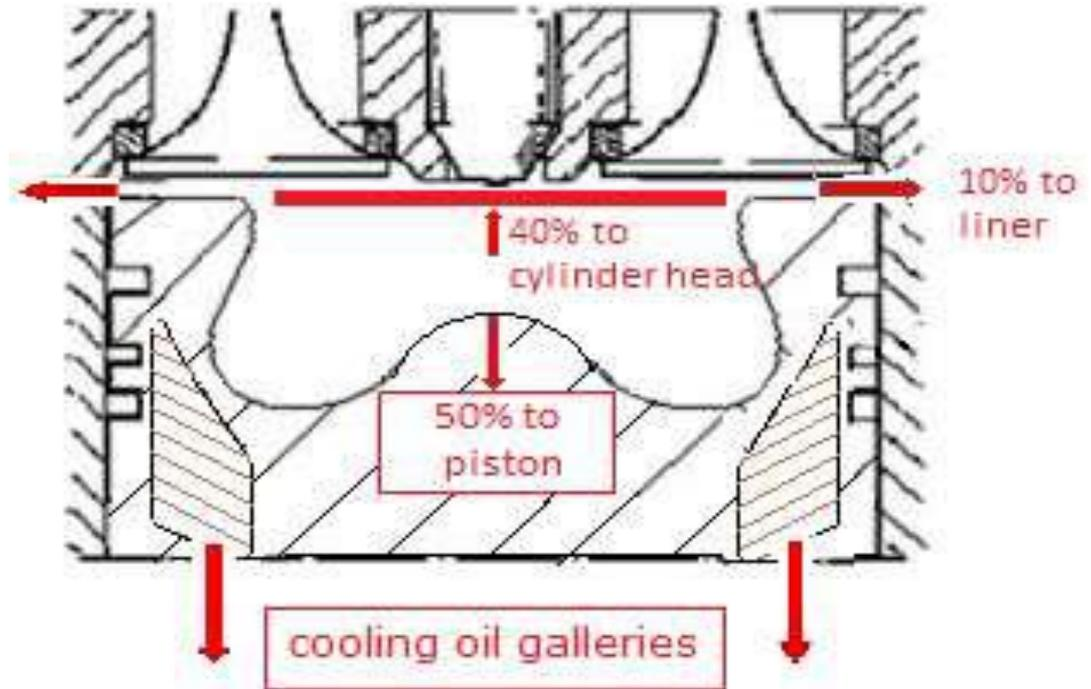
Piston head loses a high level of thermal efficiency of about 12%.
