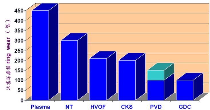
Those coatings are for reducing mechanical loss and increasing operational reliability
