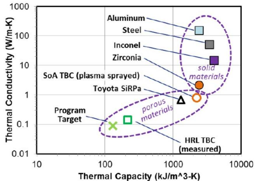
TBC must have low  $k$  and low  $c_p$  to follow the combustion gas temperature closely and reduce heat loss. This mitigates both knock tendencies and volumetric efficiency losses, unlike solid ceramic coatings with high  $c_p$ .
