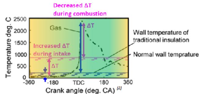
$$\dot{Q} = hA(T_{gas} - T_{wall})$$
